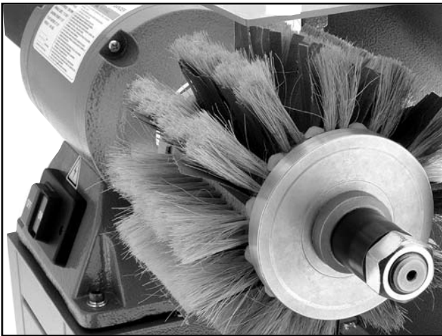
Figure 22. Correctly installed flap sander.
